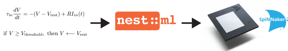
Figure 1: Workflow for formalising and simulating neuron models with NESTML and PySpiNNaker2: A mathematical model describing neuronal dynamics is formulated in the NESTML syntax by the user, after which automatic translation to C- and Python-code makes the model available for deploying SNN simulations on SpiNNaker2.
